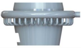
SCHEMATIC VIEW OF TUYERES AND BUSTLE PIPE
